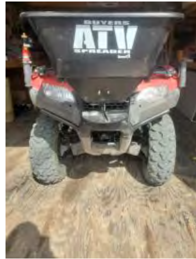
Spreader mounted on ATV
